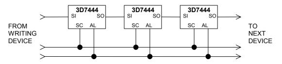
Figure 3: Cascading Multiple Devices
