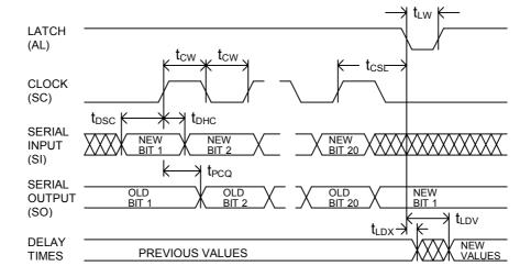
Figure 2: Serial interface timing diagram
