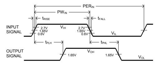
Figure 5: Timing Diagram
